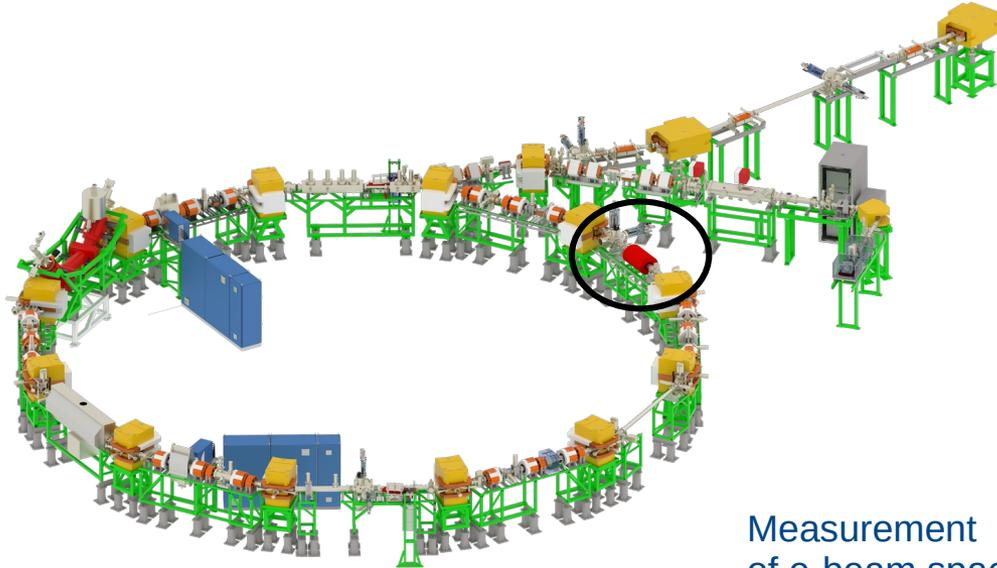
Compensation solenoid contains the **Schottky pickups** of CRYRING.
