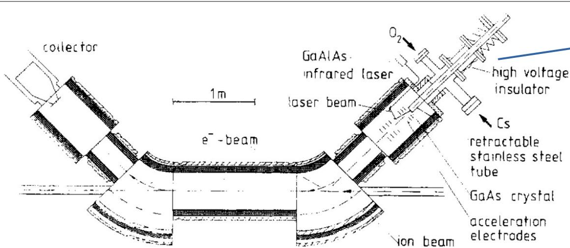
Cryogenic GaAs-photocathode e-gun
